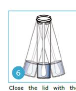
6 Close the lid with the tamper-proof cap (it will click when properly closed) and mix by shaking the tube.
