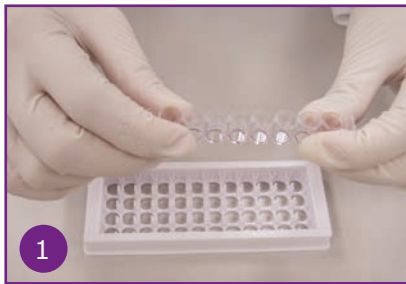
1 Break off number of wells needed and place them in the rack
