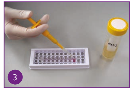
3 Add 50 µL of sample extract into each well and mix
