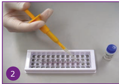
2 Pipette 50 µL of assay diluent into each wells
