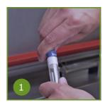
Open the swab kit by unscrewing the swab from the vial.
