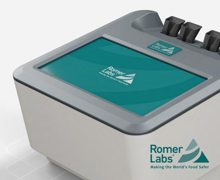
STEP 1 Turn on the AgraVision™ Pro reader by plugging the reader into an electrical socket. The screen will appear and display the Romer Labs® logo. Select the appropriate user or admin.
