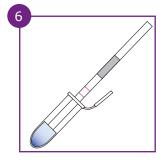
Place one test strip into the incubation vial and incubate for **5 minutes.** Remove the test strip and read the result immediately.
