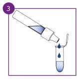
Transfer **12 drops (400 µl)** of the sample supernatant into the incubation vial by squeezing the extraction tube.
