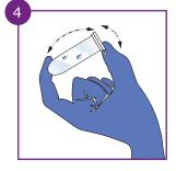
Shake the incubation vial vigorously by hand for **15 seconds** (ensuring that the liquid comes in contact with the lid of the vial).
