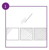
Fill one extraction tube with extraction Buffer up to where the tube gets thicker, wet the swab by dipping into the buffer. Wipe an area of 5 cm x 5 cm using side to side movements, rotating the swab tip as you qo.
